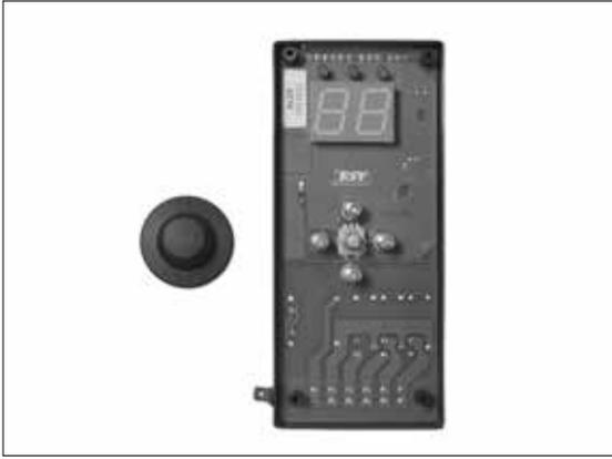
**Code: P0449** AC19 controler is designed to control boilers DCxxSR (GSR) or to control pneumatic pellet feeding system APS 250 / 500
