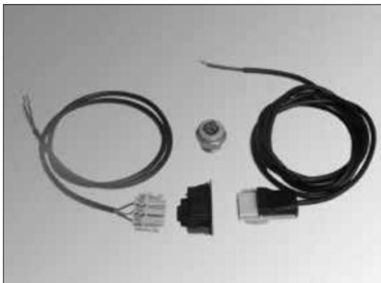
**Code: S0516** the set is for controlling pump in the primary boiler circuit by waste gas thermostat built in the dash board of the boiler. The set consists of incoming cable with connector and safety thermostat for pump 95°C
