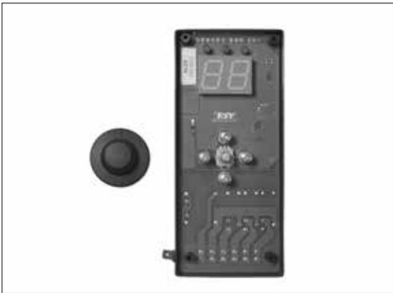
**Code: P0449** AC19 controller is designed to control pneumatic pellet feeding APS 250/500
